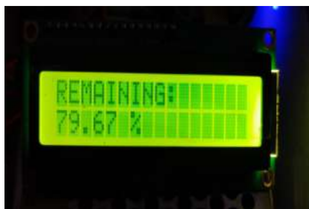
Fig.16: The remaining level of the IV drip which will display after the flow begins.
